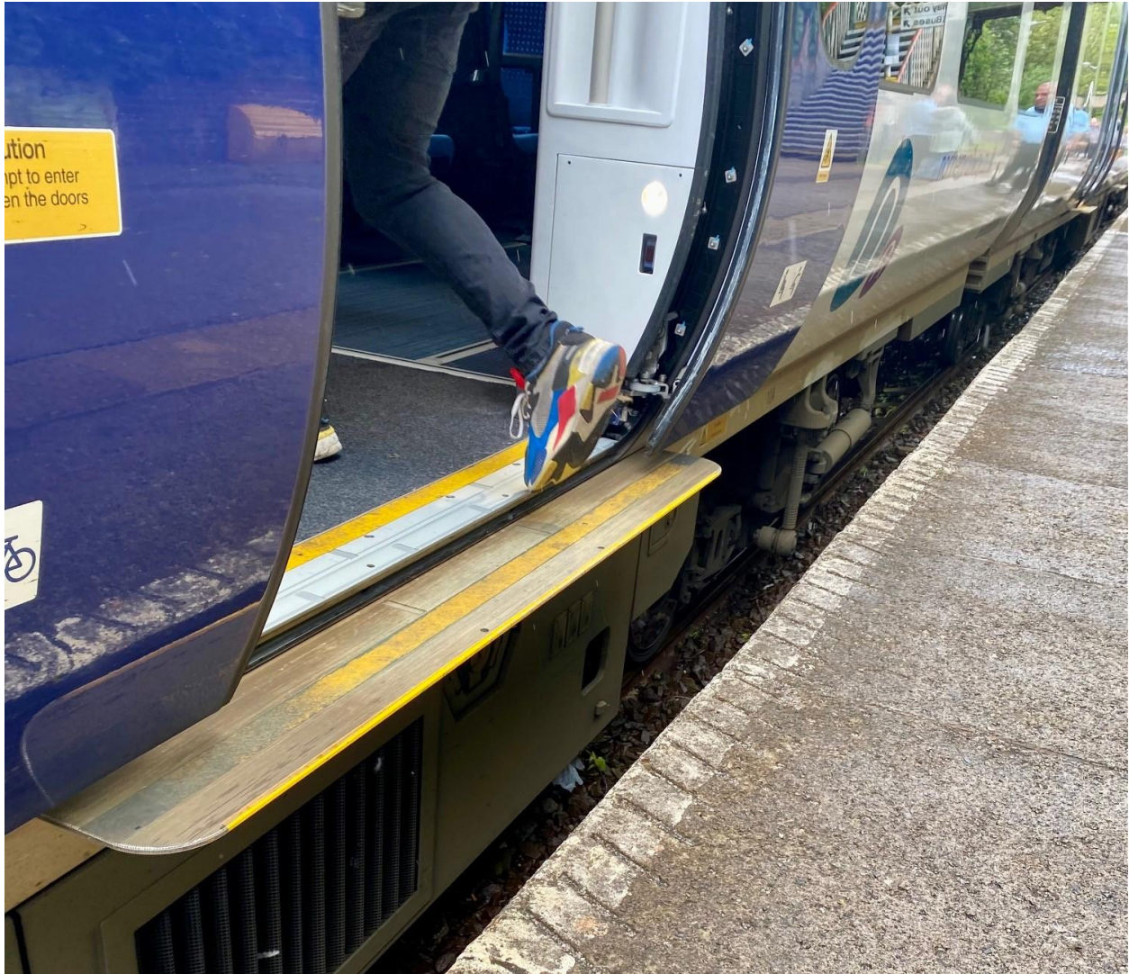
Photo: the large gap between the train and platform at a Northern operated station. The large gaps can make it very difficult for parents, especially solo parents, travelling with a young child in a buggy to get on and off the train safely. (Credit: Campaign for Family Friendly Trains)
