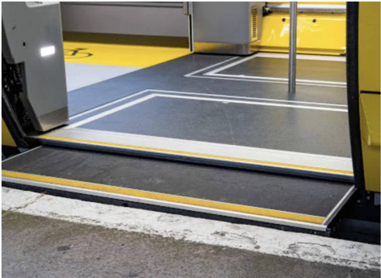
Photo: Merseyrail's new fleet of trains have a sliding step which allows level boarding from platform to train at all stations in the operator's network (Credit: Merseyrail)
